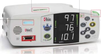
The System Status Indicator: provides a visual indication of alarm and data-collection alerts, even when parameter display screen is not visible to clinician.
