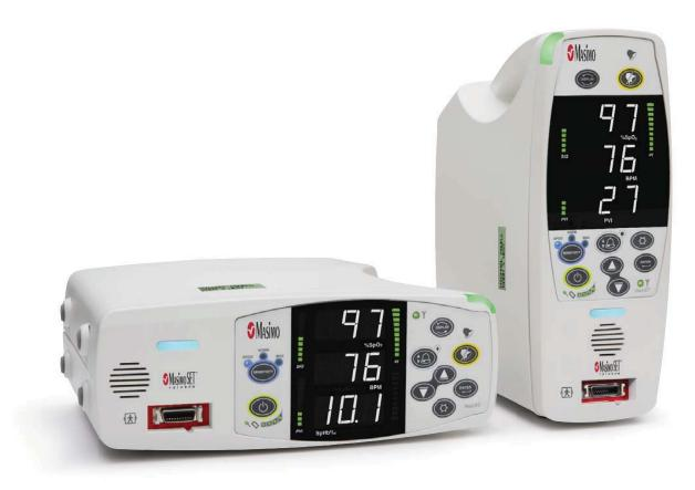
Choose the noninvasive measurements that are right for your clinical setting—oxygen saturation, pulse rate, and perfusion index in addition to total hemoglobin, total arterial oxygen content, PVI, carboxyhemoglobin, and methemoglobin
